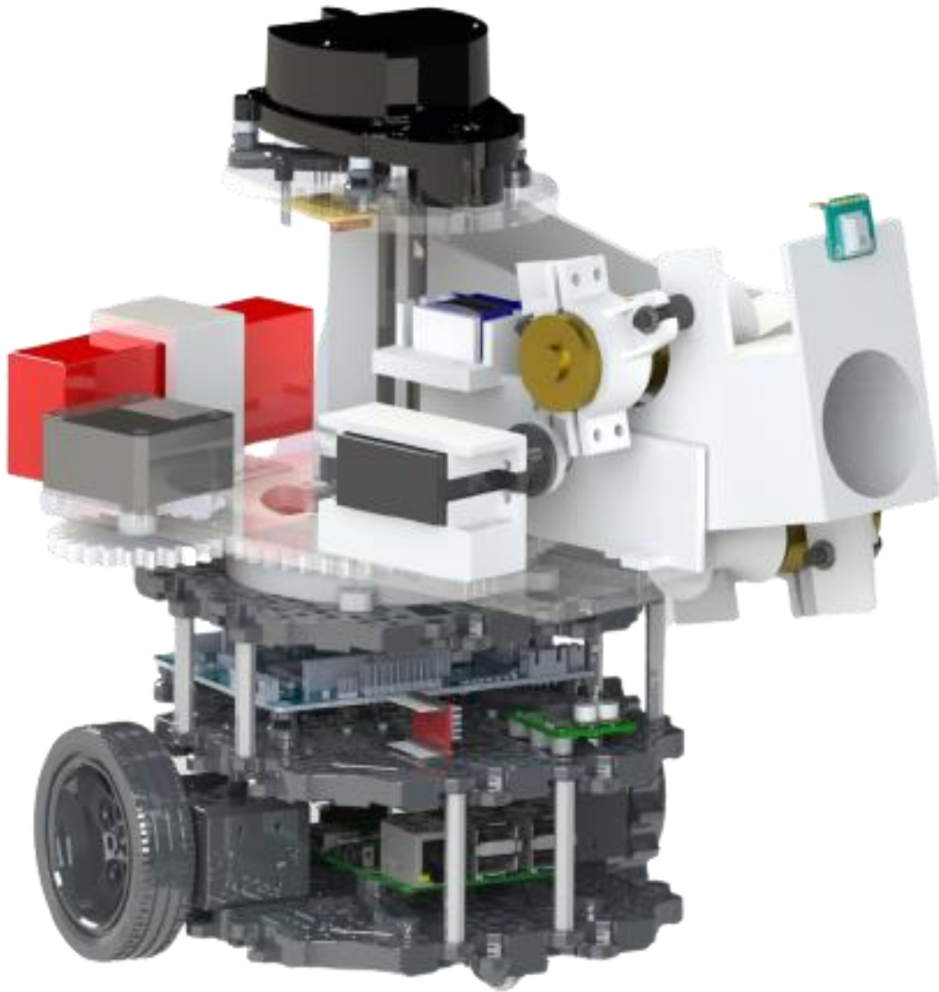
Figure 38: Render of how the final assembled A.N.T. should look
