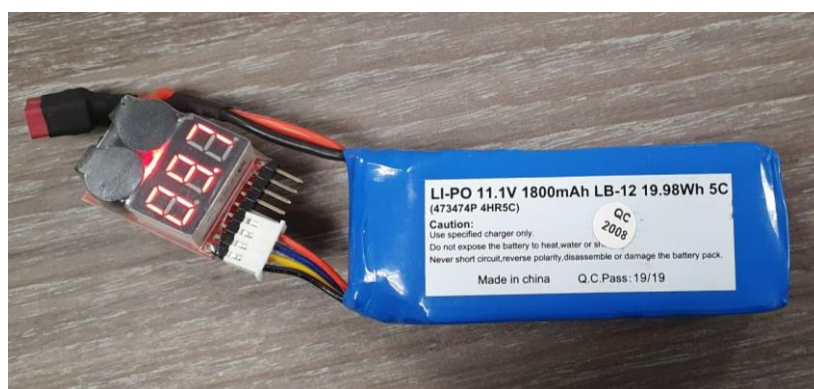
Figure 45: Battery Connected to Battery Voltage Checker
