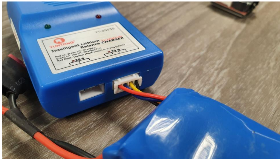
Figure 44: Battery Connected to Charger Properly
